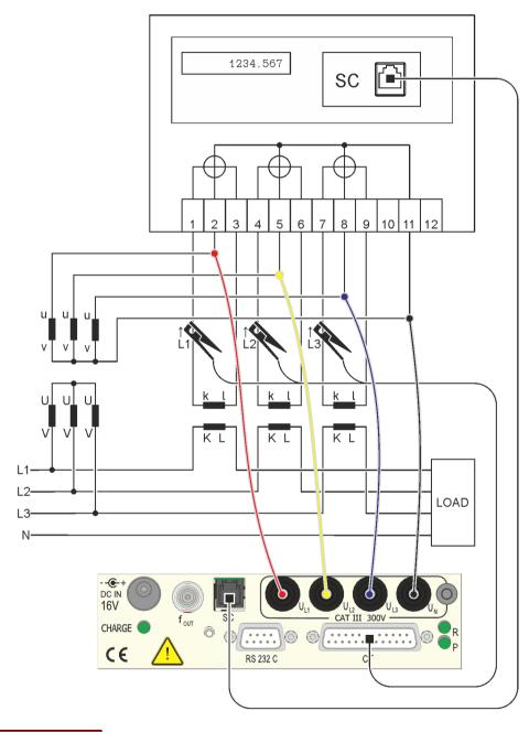
Do not open the secondary side of the current transformer
