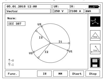
Options 'DIN 410': U1 vertically upwards is defined as  $\varphi = 0$ .
