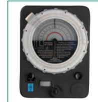
An electromechanical fault indicator type FA3, used to test a dynamic meter. The difference between the set and actual time can be directly read off the dial.
