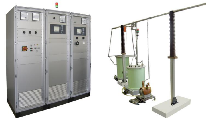
ITTS (CT-VT-80) CT and VT Test System Generation: max. 80 kVA
