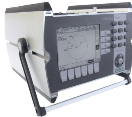
MT500 Current and voltage source 12 A / 300 V
