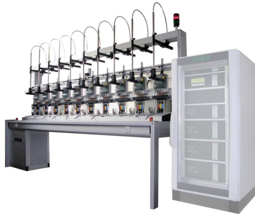
Multi-Position Test Bench 5, 10, 20 or 40 test positions different designs
